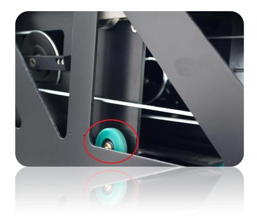
To tune up the green wheel you need to loose (don't release it) the helical screw...
