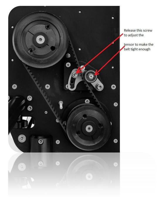
**A.4.** How to tension the cables.
