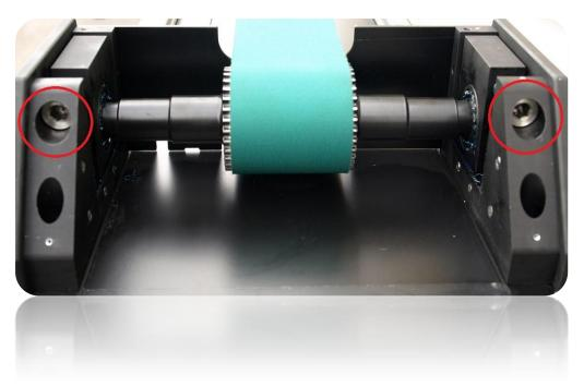
Strain the upper belt when the crane is fully loaded and shorten to maximum at maximum angle. In that position the belt is in its heaviest working conditions. The belt cannot slide on the section at that time.
