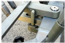
Switch lever (here in upward position)
