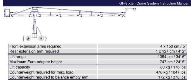
Crane weight (excluding dolly and weights)217 kg / 477 lbsDolly weight80 kg / 176 lbsArm reach (pivot to camera head mount)713 cm / 23' 4"Length of rear end (pivot to outside of bucket)220 cm / 7' 2"
