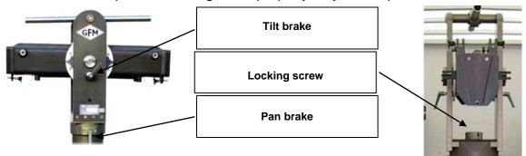
Middle section with pan and tilt lock
