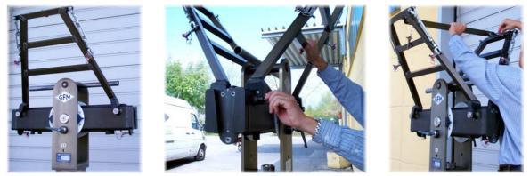
7. For Standard Versions 1 to 16 connect the 127cm / 4ft rear arm section to the middle section. For Standard Versions 17 and 18 connect the 150cm / 5ft section to the middle section. Slip the connection flanges into each other and secure with the provided safety pin.
