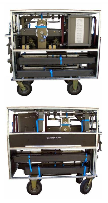
The above photos show the practical transport solution for the GF-8 Crane System. The GFM trolley fits the complete system with dolly and column as an extra unit.
