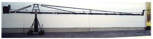
Attention: The rigging system of the crane arm should be hand tightened symmetrically from both sides of the crane in a way that the arm is absolutely straight when carrying the loads of the counterweight bracket, the platform or remote bracket.
